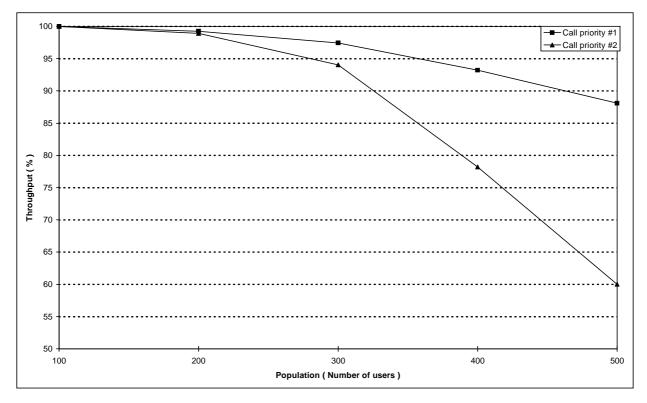
Figure 174: Individual M-M circuit switched call set-up system throughput versus number of users for priority distribution C
