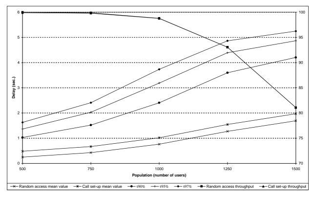
Figure 88: Individual M-F short data transmission performance for scenario 1B (throughput curves overlap)
