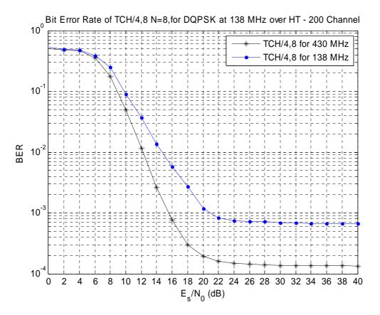
Figure F.26: Bit Error Rate of TCH/4,8 N=8 over HT200 Propagation Channel for 138 MHz
