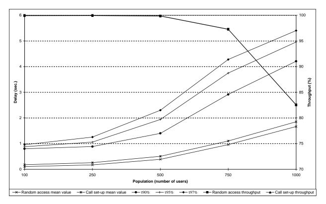
Figure 89: Individual M-M voice or circuit data call performance for scenario 1C (throughput curves overlap)
