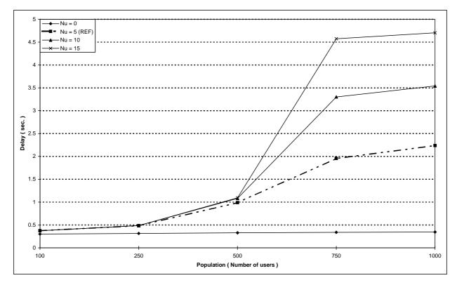
Figure 110: Individual M-F short data transmission mean delay versus number of users for different values of the maximum number of re-transmissions in the random access Nu
