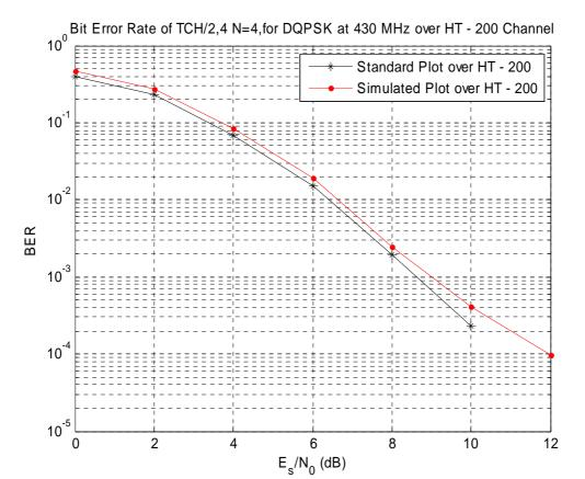
Figure G.19: Bit Error Rate of TCH/2,4 N=4 Channel over HT200 propagation channel for 430 MHz, results corresponds to figure 59 of clause 4.4
