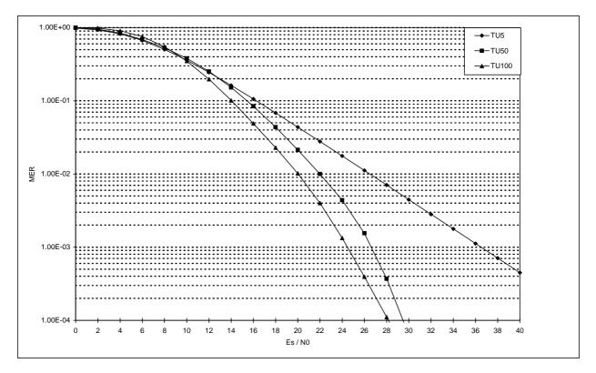
Figure 15: Influence of MS speed on SCH/F in TU propagation environment
