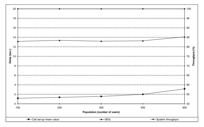
Figure 167: Individual M-M packet data call set-up performance versus number of users for priority distribution A
