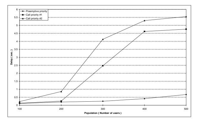
Figure 169: Individual M-M circuit switched call set-up  $\tau_{95\%}$  boundary delay versus number of users for priority distribution B
