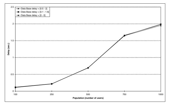
Figure 78: Comparison of random access mean value for different characteristics of system data base (all curves overlap)
