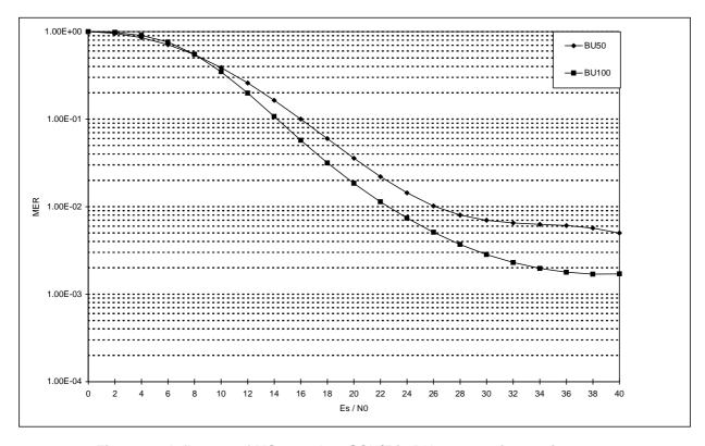
Figure 16: Influence of MS speed on SCH/F in BU propagation environment
