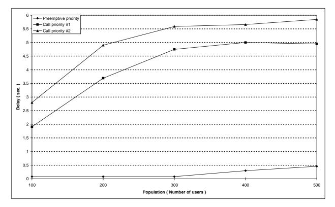
Figure 184: Individual M-M circuit switched call set-up  $\tau_{95\%}$  boundary delay versus number of users in a cell with 3 TCHs allocated
