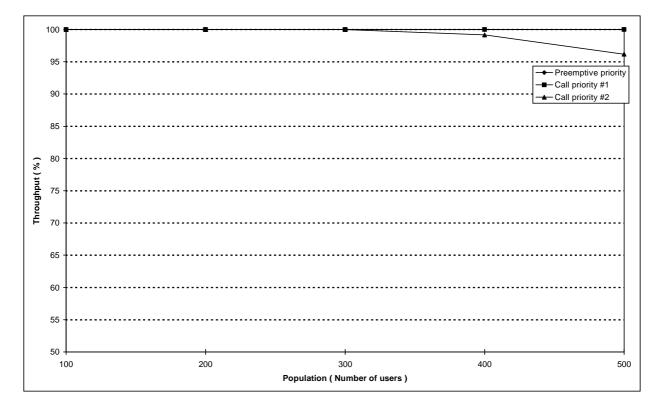
Figure 189: Individual M-M circuit switched call set-up system throughput versus number of users in a cell with 11 TCHs allocated
