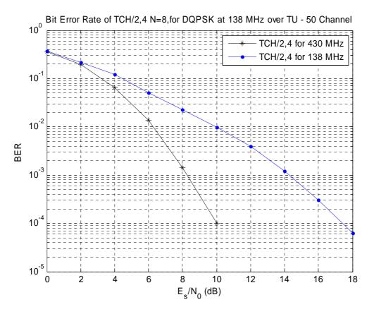
Figure F.12: Bit Error Rate of TCH/2,4 N=8 over TU50 Propagation Channel for 138 MHz
