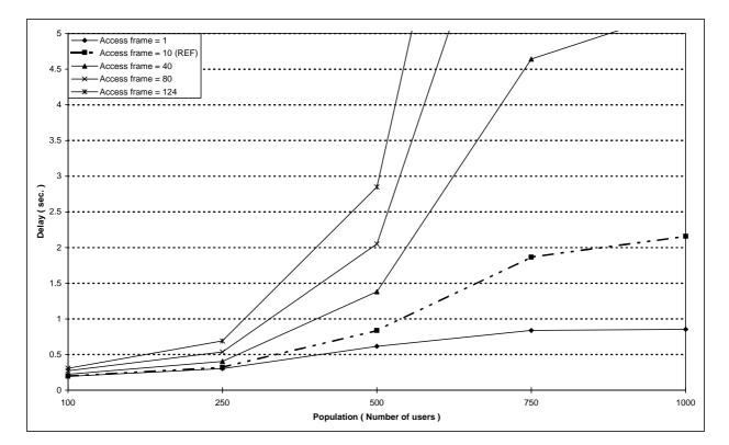
Figure 115: Individual M-M circuit switched call set-up mean delay versus number of users for different values of the random access frame length
