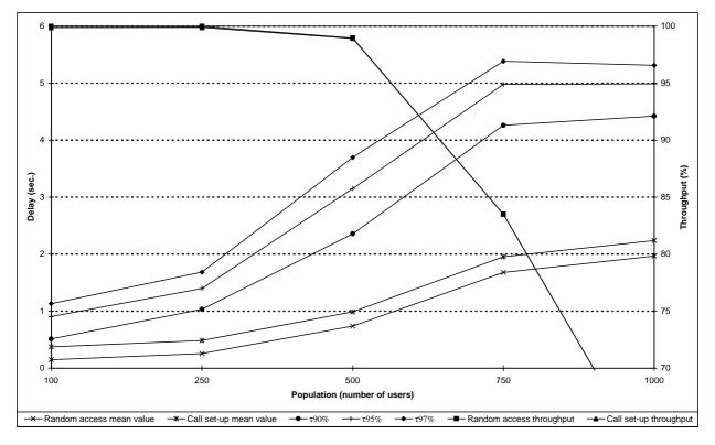
Figure 92: Individual M-F short data transmission performance for scenario 1D (reference) (throughput curves overlap)
