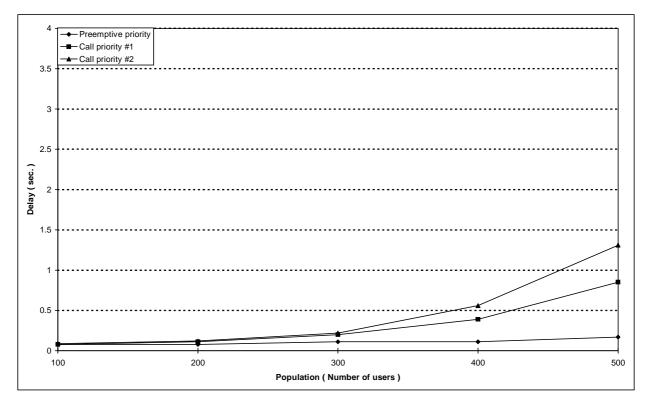
Figure 160: Individual M-M circuit switched call set-up mean delay versus number of users for scenario 8E (No Dispatcher)
