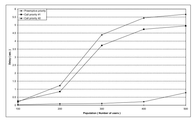
Figure 158: Dispatcher to Mobile group call set-up  $\tau_{95\%}$  boundary delay versus number of users for the reference configuration
