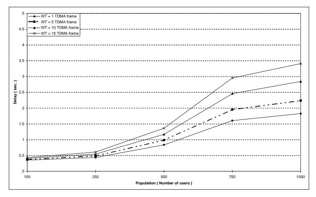
Figure 102: Individual M-F short data transmission mean delay versus number of users for different values of the retransmission timer WT
