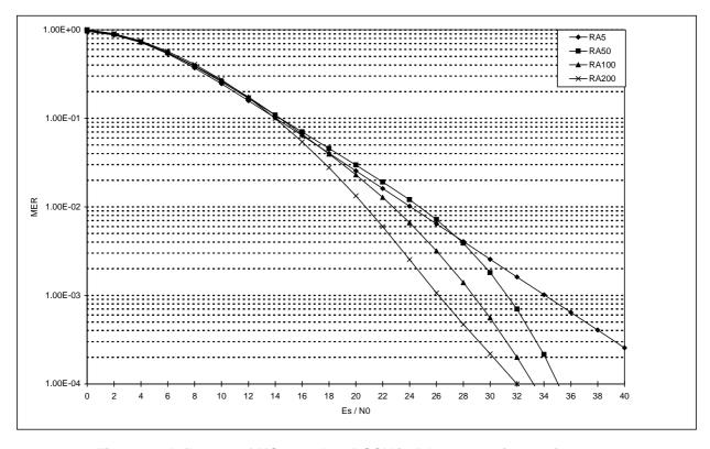
Figure 23: Influence of MS speed on BSCH in RA propagation environment
