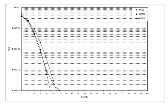
Figure 65: Influence of MS speed on TCH/2,4 N=8 in HT propagation environment
