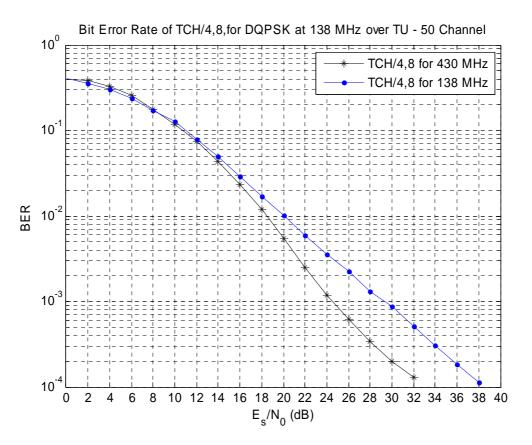
Figure F.13: Bit Error Rate of TCH/4,8 over TU50 Propagation Channel for 138 MHz
