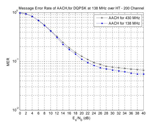
Figure F.16: Message Error Rate of AACH over HT200 Propagation Channel for 138 MHz
