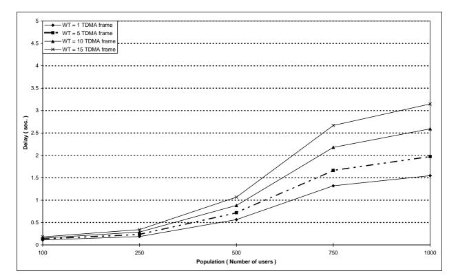
Figure 97: Random access mean delay versus number of users for different values of the retransmission timer WT
