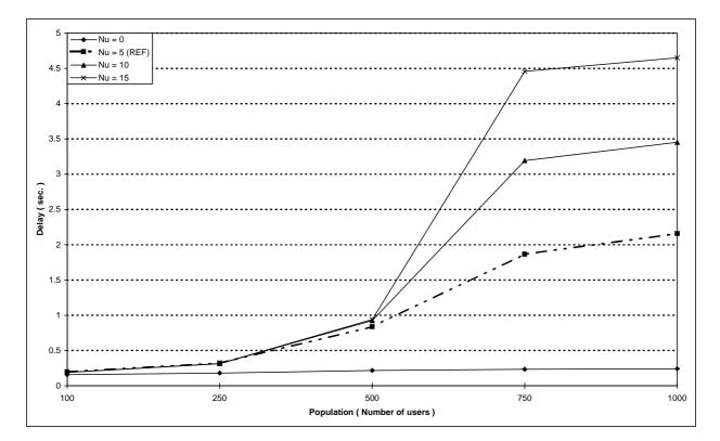
Figure 107: Individual M-M circuit switched call set-up mean delay versus number of users for different values of the maximum number of re-transmissions in the random access Nu
