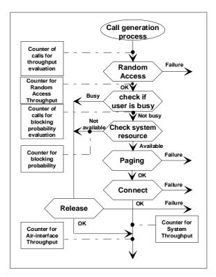
Figure 73: Group circuit call procedure scheme with counters for the evaluation of throughput parameters
