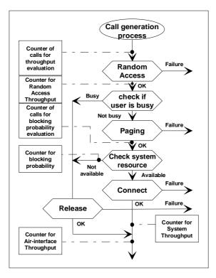
Figure 72: Individual circuit call procedure scheme with counters for the evaluation of throughput parameters
