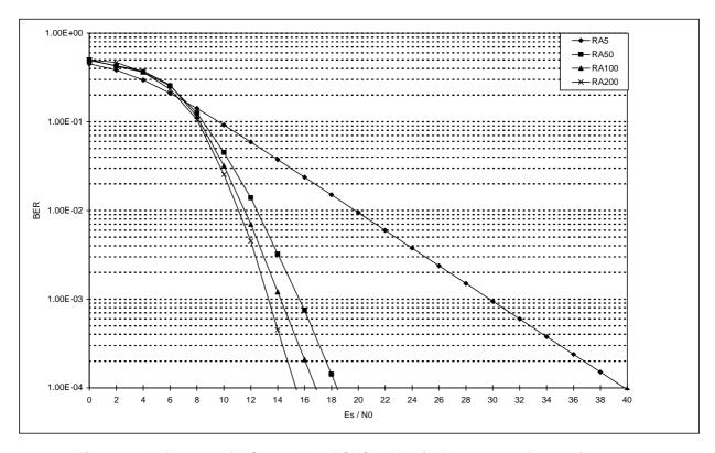
Figure 40: Influence of MS speed on TCH/4,8 N=4 in RA propagation environment
