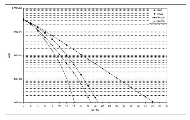
Figure 52: Influence of MS speed on TCH/2,4 N=1 in RA propagation environment
