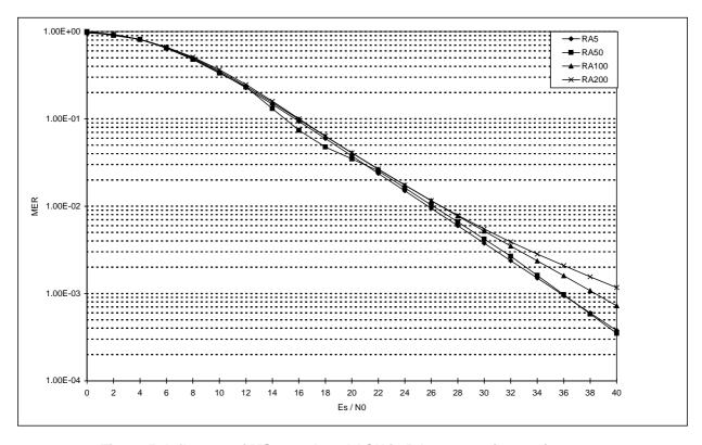
Figure 5: Influence of MS speed on AACH in RA propagation environment
