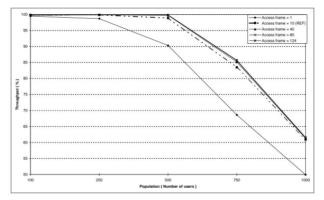
Figure 119: Individual M-F short data transmission throughput versus number of users for different values of the random access frame length
