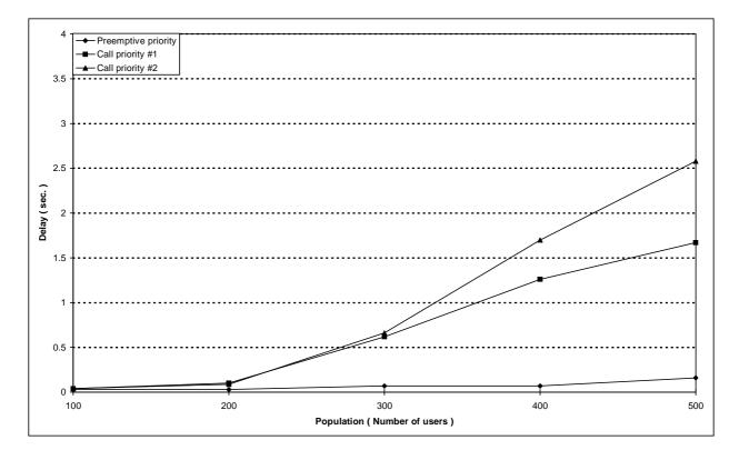
Figure 157: Dispatcher to Mobile group voice call set-up mean delay versus number of users for the reference configuration
