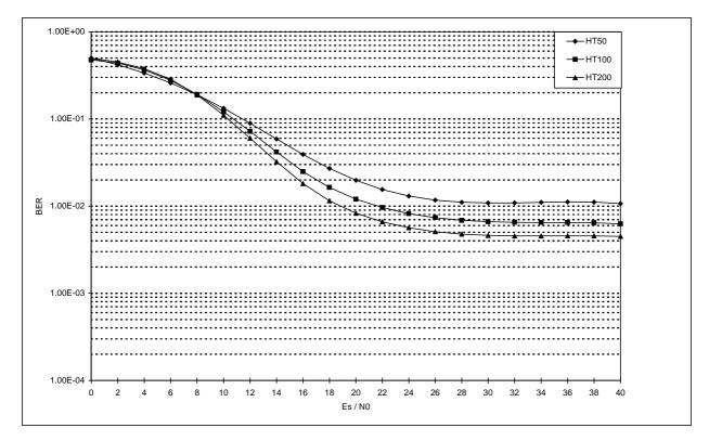
Figure 35: Influence of MS speed on TCH/4,8 N=1 in HT propagation environment
