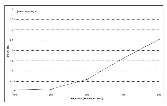
Figure 164: Individual M-M circuit switched call set-up mean delay versus number of users for priority distribution A
