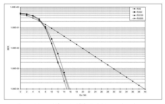
Figure 46: Influence of MS speed on TCH/4,8 N=8 in RA propagation environment
