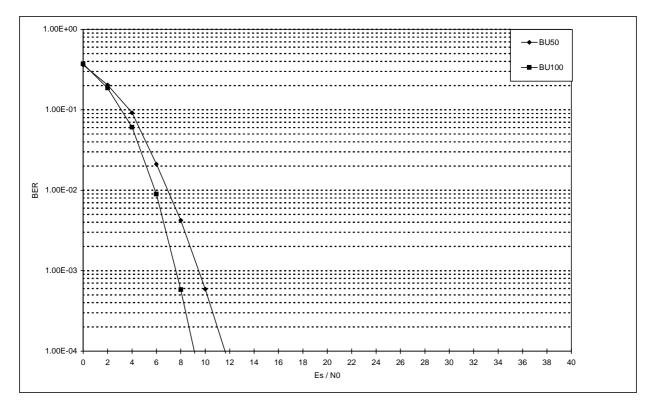
Figure 63: Influence of MS speed on TCH/2,4 N=8 in BU propagation environment
