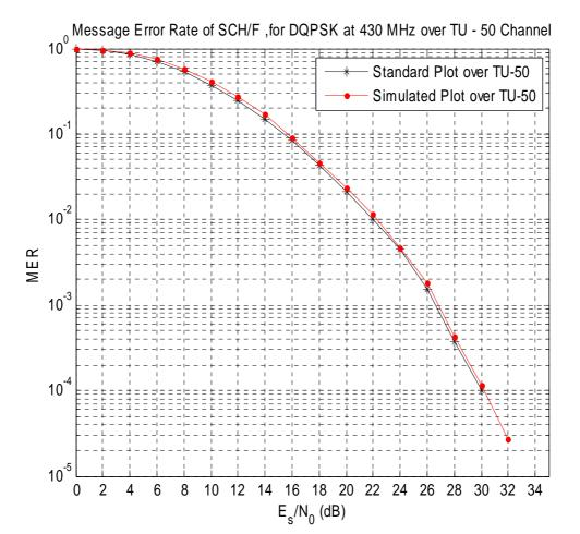
Figure G.4: Message Error Rate of SCH/F over TU-50 propagation channel for 430 MHz, results corresponds to figure 15 of clause 4.3
