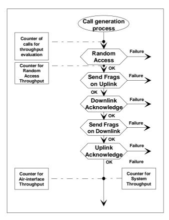
Figure 74: Packet data call procedure scheme with counters for the evaluation of throughput parameters
