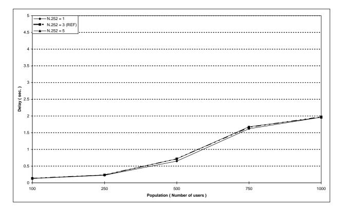
Figure 121: Random access mean delay versus number of users for different values of the basic link maximum number of re-transmissions
