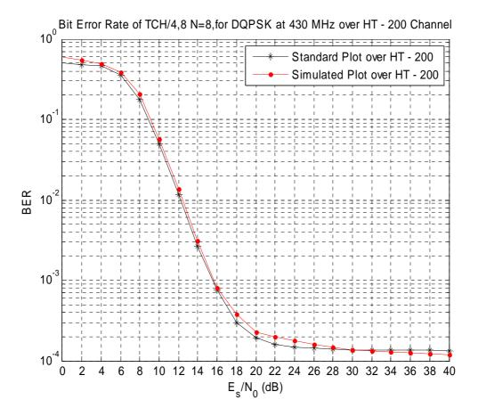
Figure G.22: Bit Error Rate of TCH/4,8 N=8 Channel over HT200 propagation channel for 430 MHz, results corresponds to figure 47 of clause 4.4
