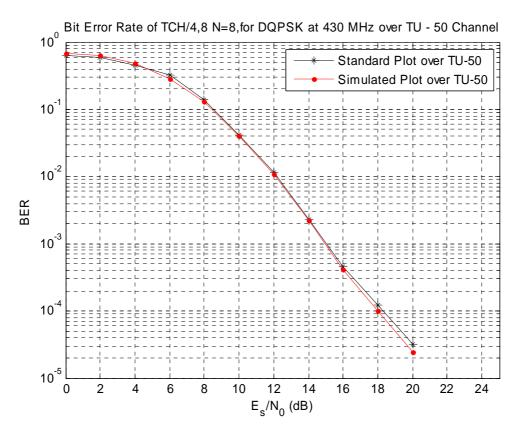
Figure G.12: Bit Error Rate of TCH/4,8 N=8 over TU50 Propagation Channel for 430 MHz, results corresponds to figure 44 of clause 4.4
