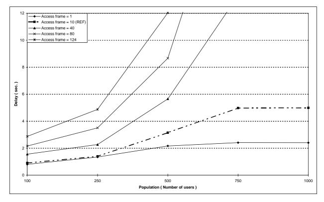
Figure 120: Individual M-F short data transmission  $\tau_{95\,\%}$  boundary delay versus number of users for different values of the random access frame length
