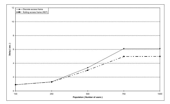
Figure 133: Individual M-M circuit switched call set-up  $\tau_{95\%}$  boundary delay versus number of users for different access techniques
