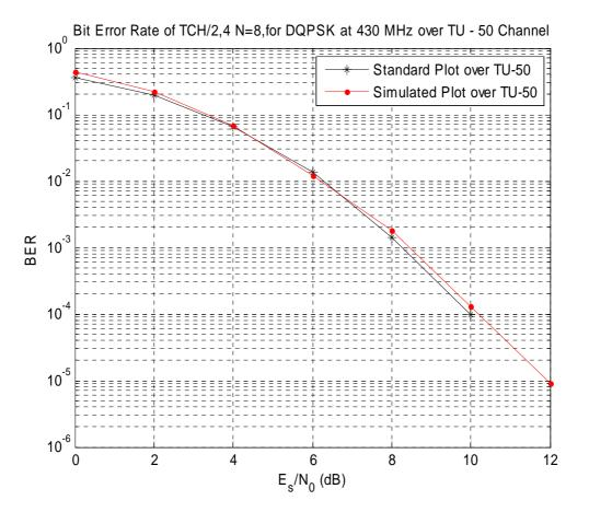
Figure G.9: Bit Error Rate of TCH/2,4 N=8 over TU50 propagation channel for 430 MHz, results corresponds to figure 62 of clause 4.4
