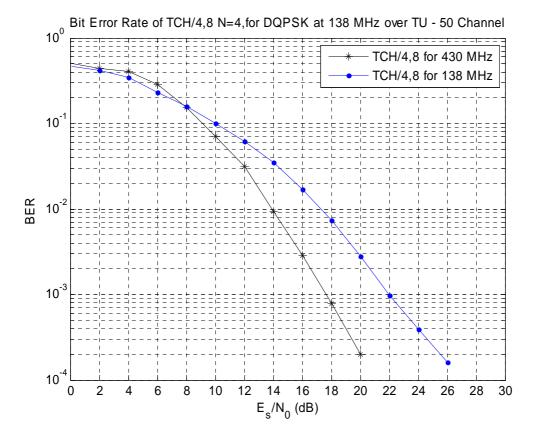
Figure F.14: Bit Error Rate of TCH/4,8 N=4 over TU50 Propagation Channel for 138 MHz
