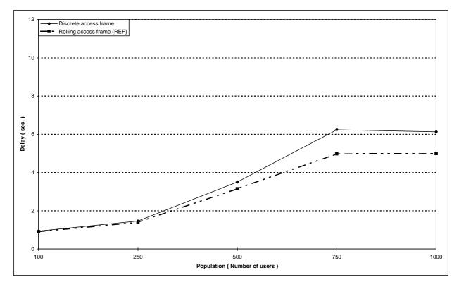
Figure 136: Individual M-F short data transmission  $\tau_{95\%}$  boundary delay versus number of users for different access techniques
