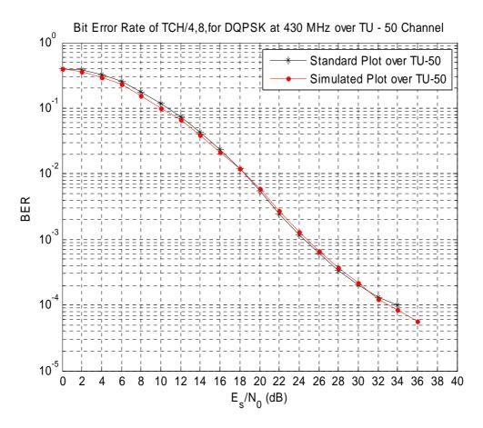
Figure G.10: Bit Error Rate of TCH/4,8 over TU50 propagation channel for 430 MHz, results corresponds to figure 32 of clause 4.4
