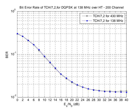
Figure F.20: Bit Error Rate of TCH/7,2 over HT200 Propagation Channel for 138 MHz
