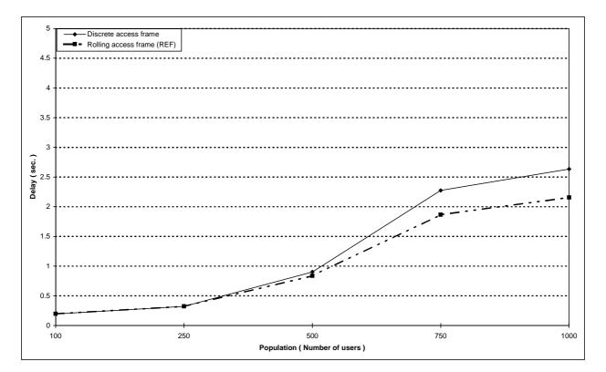
Figure 131: Individual M-M circuit switched call set-up mean delay versus number of users for different access techniques
