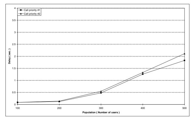
Figure 172: Individual M-M circuit switched call set-up mean delay versus number of users for priority distribution C
