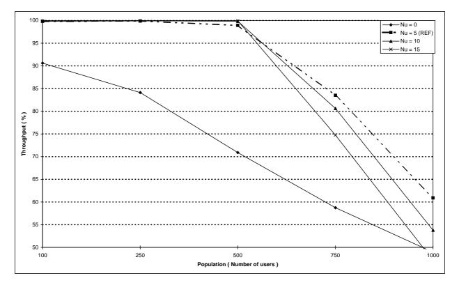
Figure 111: Individual M-F short data transmission throughput versus number of users for different values of the maximum number of re-transmissions in the random access Nu
