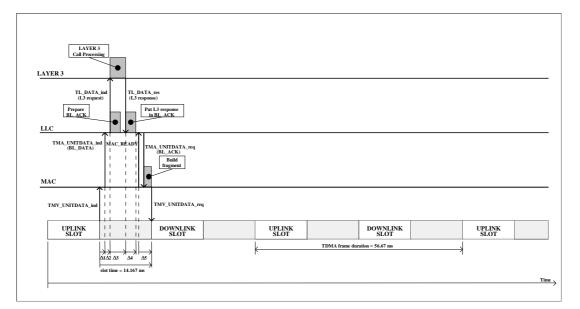
Figure 68: Time diagram related to message exchange in MAC, LLC and layer 3 with short response times
