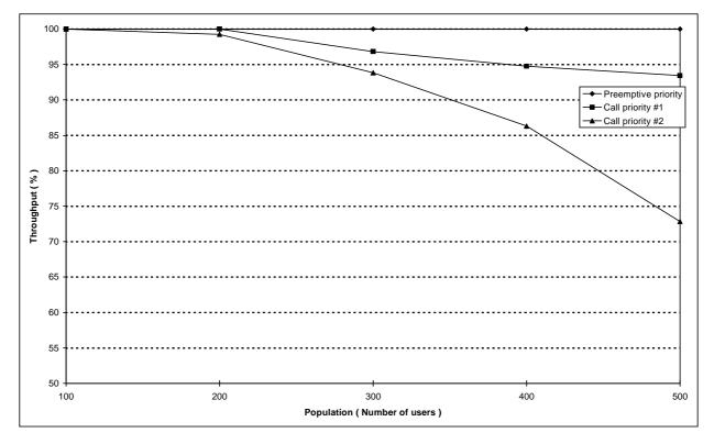
Figure 144: Dispatcher to Mobile group voice call set-up system throughput versus number of users for the reference scenario
