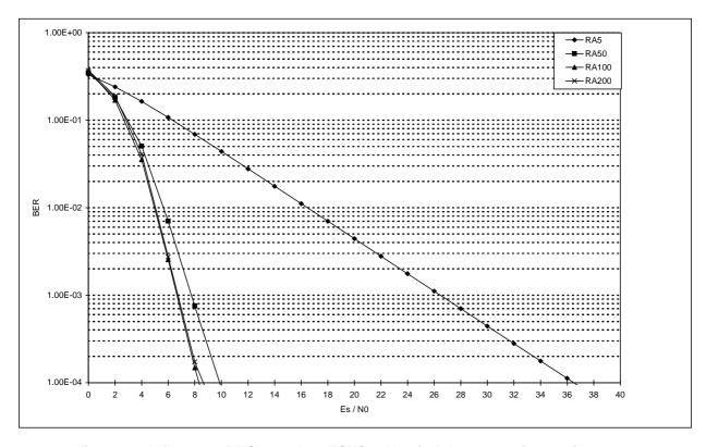
Figure 64: Influence of MS speed on TCH/2,4 N=8 in RA propagation environment
