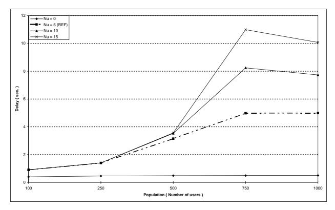
Figure 112: Individual M-F short data transmission  $\tau_{95\%}$  boundary delay versus number of users for different values of the maximum number of re-transmissions in the random access Nu
