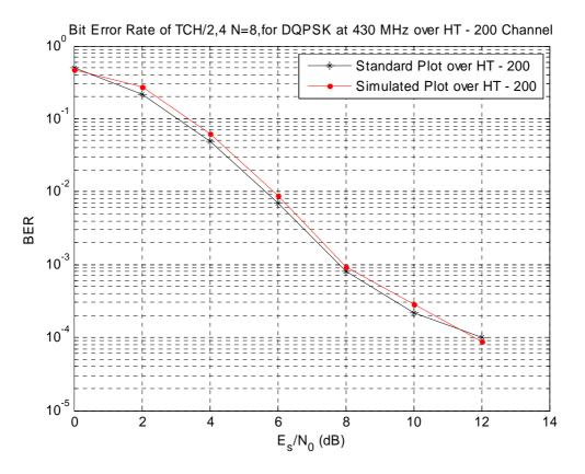
Figure G.20: Bit Error Rate of TCH/2,4 N=8 Channel over HT200 propagation channel for 430 MHz, results corresponds to figure 65 of clause 4.4
