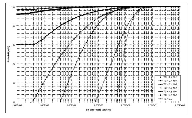
Figure 201: BER versus probability for different traffic channels in RA 50 propagation environment
