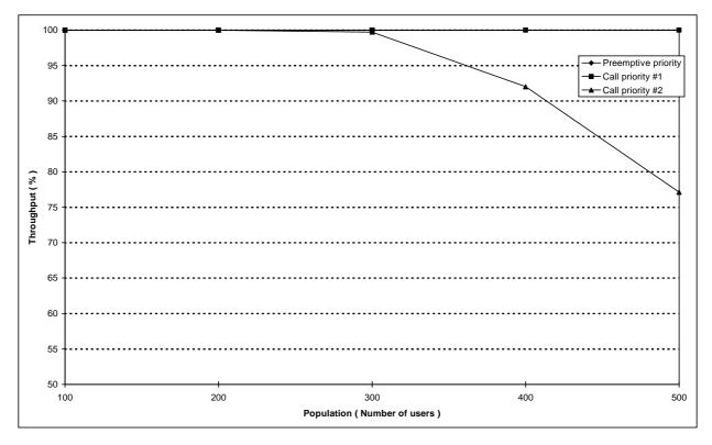
Figure 193: Individual M-M circuit switched call set-up system throughput versus number of users with maximum hold time in priority queue = 300 TDMA frames
