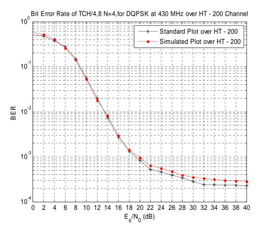
Figure G.27: Bit Error Rate of TCH/4,8 N=4 Channel over HT200 propagation channel for 430 MHz, results corresponds to figure 41 of clause 4.4
