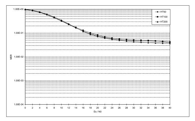
Figure 24: Influence of MS speed on BSCH in HT propagation environment
