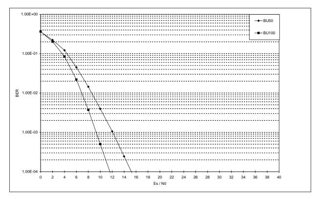
Figure 57: Influence of MS speed on TCH/2,4 N=4 in BU propagation environment
