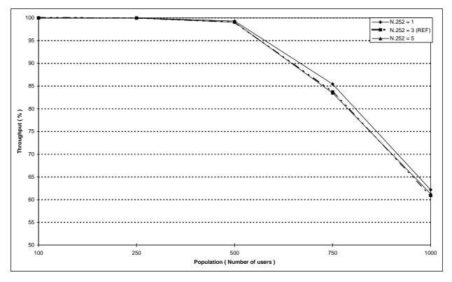
Figure 122: Random access throughput versus number of users for different values of the basic link maximum number of re-transmissions
