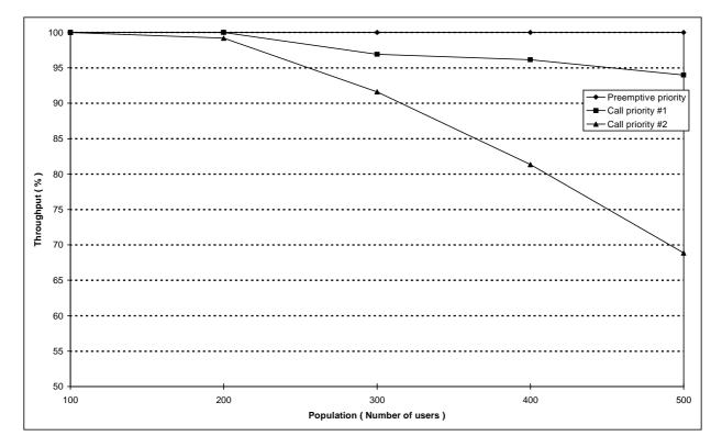
Figure 155: Individual M-M circuit switched call set-up system throughput versus number of users for scenario 8D (Reference with radio Dispatcher)
