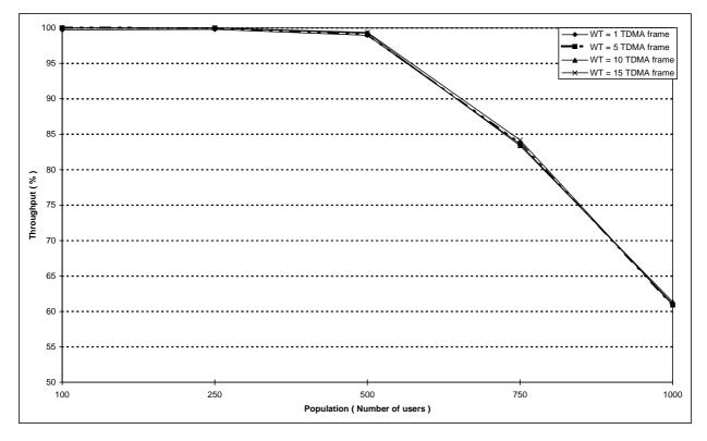
Figure 98: Random access throughput versus number of users for different values of the retransmission timer WT (all curves overlap)
