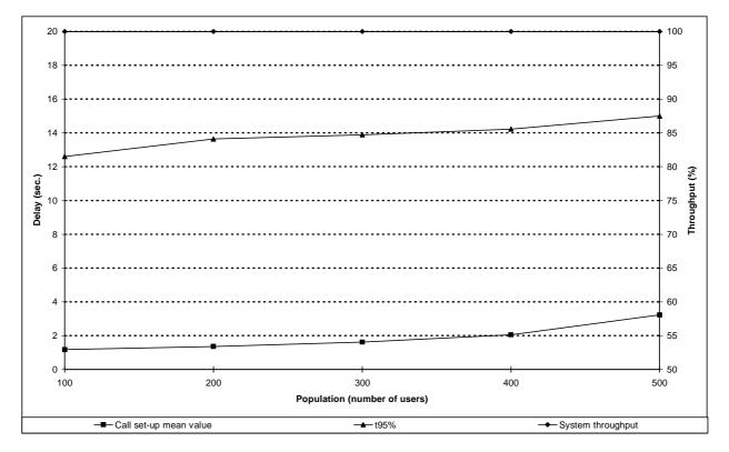
Figure 194: Individual M-M packet data call set-up performance versus number of users with maximum hold time in priority queue = 300 TDMA frames
