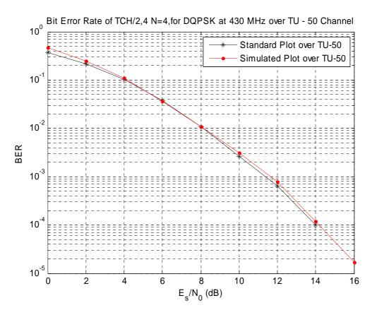
Figure G.8: Bit Error Rate of TCH/2,4 N=4 over TU50 propagation channel for 430 MHz, results corresponds to figure 56 of clause 4.4
