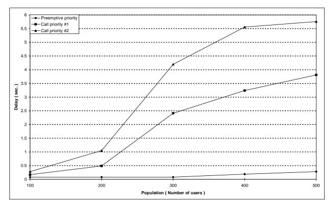
Figure 146: Individual M-M circuit switched call set-up  $\tau_{95\%}$  boundary delay versus number of users for scenario 8B (Packet data generation rate = 15/h)
