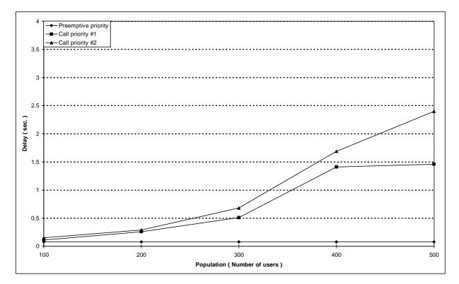
Figure 149: Individual M-M circuit switched call set-up mean delay versus number of users for scenario 8C (Packet data generation rate = 30/h)
