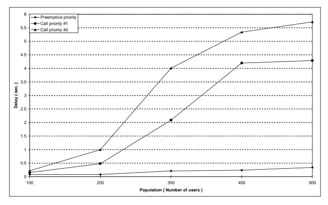
Figure 154: Individual M-M circuit switched call set-up  $\tau_{95\%}$  boundary delay versus number of users for scenario 8D (Reference with radio Dispatcher)
