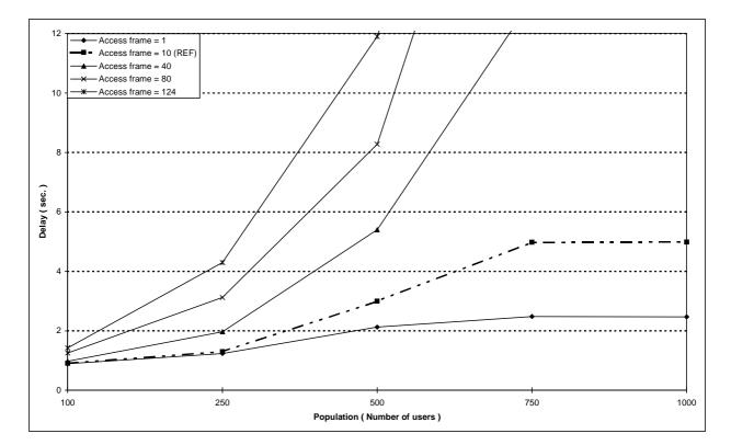
Figure 117: Individual M-M circuit switched call set-up  $\tau_{95\%}$  boundary delay versus number of users for different values of the random access frame length
