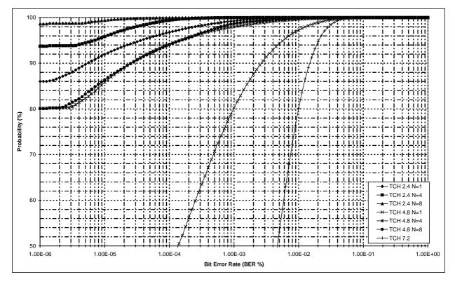
Figure 203: BER versus probability for different traffic channels in RA200 propagation environment
