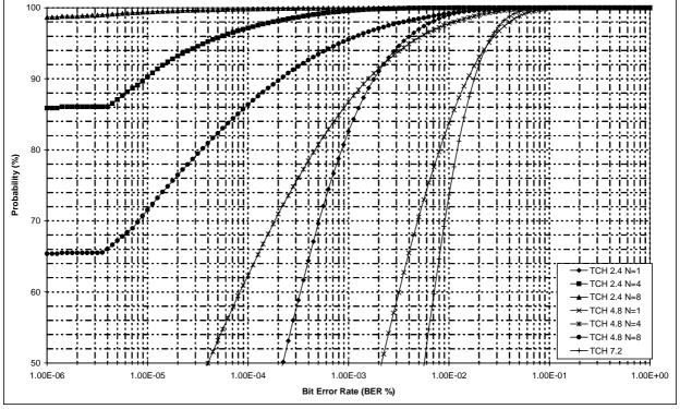
Figure 196: BER versus probability for different traffic channels in TU50 propagation environment
