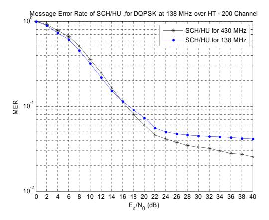
Figure F.19: Message Error Rate of SCH/HU over HT200 Propagation Channel for 138 MHz
