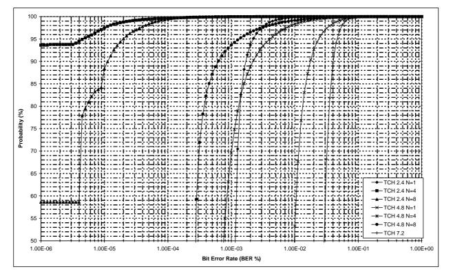
Figure 206: BER versus probability for different traffic channels in HT200 propagation environment
