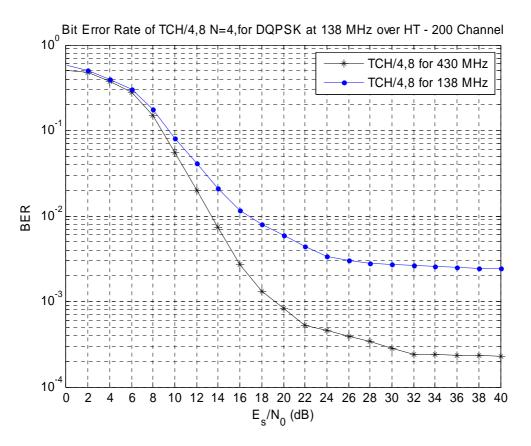
Figure F.25: Bit Error Rate of TCH/4,8 N=4 over HT200 Propagation Channel for 138 MHz
