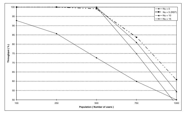
Figure 106: Random access throughput versus number of users for different values of the maximum number of re-transmissions in the random access Nu
