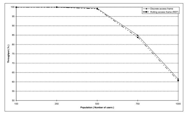
Figure 132: Individual M-M circuit switched call set-up throughput versus number of users for different access techniques
