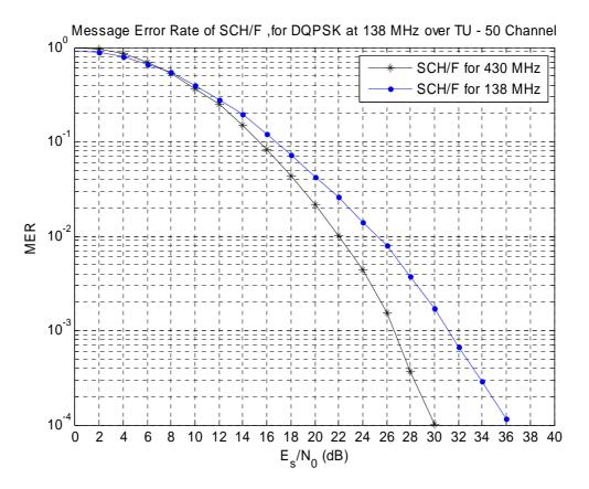
Figure F.7: Message Error Rate of SCH/F over TU50 Propagation Channel for 138 MHz
