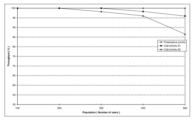
Figure 162: Individual M-M circuit switched call set-up system throughput versus number of users for scenario 8E (No Dispatcher)
