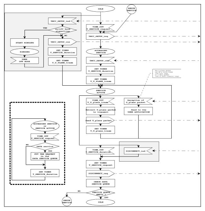
Figure C.1: SDL diagram of the user model
