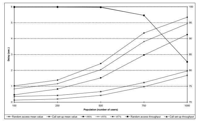
Figure 90: Individual M-F short data transmission performance for scenario 1C (throughput curves overlap)
