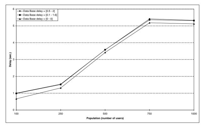
Figure 82: Comparison of call set-up τ<sub>97 %</sub> for different characteristics of system data base (curves for delay in 0,5 s to 2 s and in 0,1 s to 1,6 s overlap)
