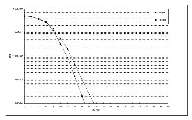
Figure 45: Influence of MS speed on TCH/4,8 N=8 in BU propagation environment
