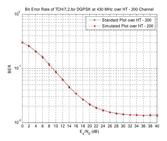
Figure G.17: Bit Error Rate of TCH/7,2 Channel over HT200 propagation channel for 430 MHz, results corresponds to figure 29 of clause 4.4
