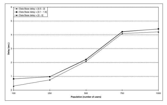
Figure 80: Comparison of call set-up  $\tau_{90\%}$  for different characteristics of system data base (curves for delay in 0,5 s to 2 s and in 0,1 s to 1,6 s overlap)
