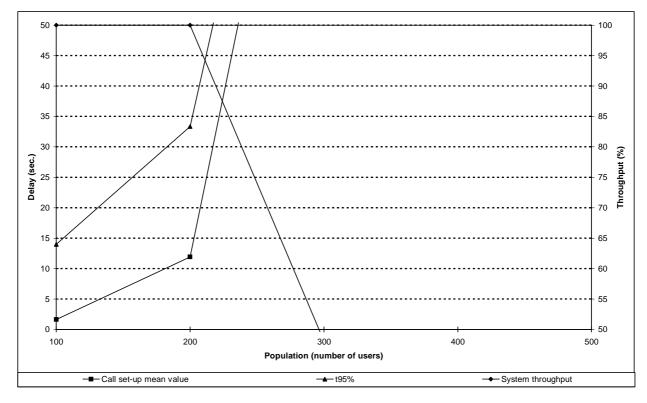
Figure 152: Individual M-M packet data call set-up performance versus number of users for scenario 8C (Packet data generation rate = 30/h)
