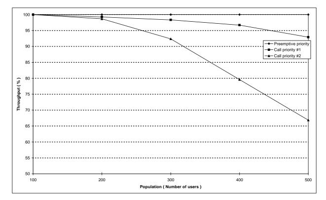
Figure 159: Dispatcher to Mobile group voice call set-up system throughput versus number of users for the reference scenario
