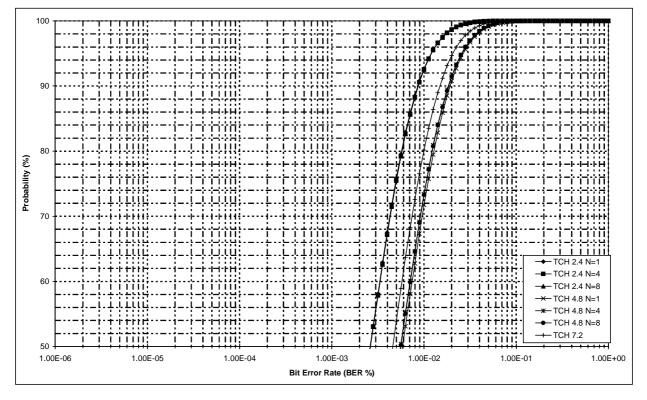
Figure 200: BER versus probability for different traffic channels in RA 5 propagation environment
