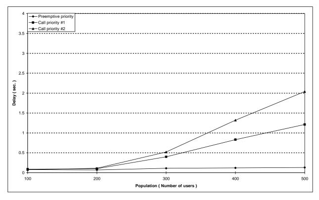
Figure 142: Dispatcher to Mobile group voice call set-up mean delay versus number of users for the reference configuration
