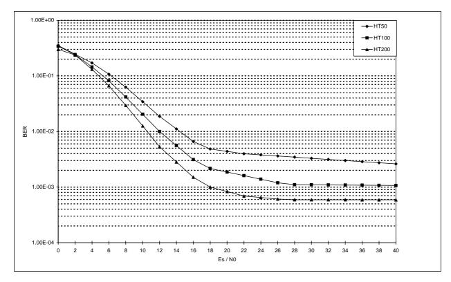
Figure 53: Influence of MS speed on TCH/2,4 N=1 in HT propagation environment
