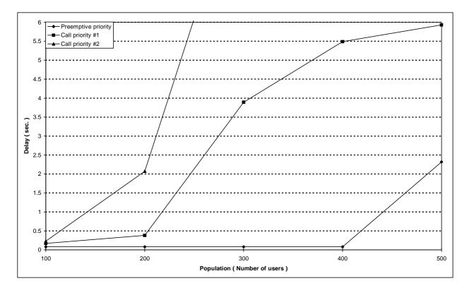
Figure 192: Individual M-M circuit switched call set-up  $\tau_{95\%}$  boundary delay versus number of users with maximum hold time in priority queue = 300 TDMA frames
