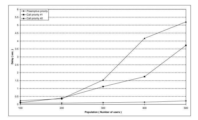
Figure 161: Individual M-M circuit switched call set-up  $\tau_{95\%}$  boundary delay versus number of user for scenario 8E (No Dispatcher)
