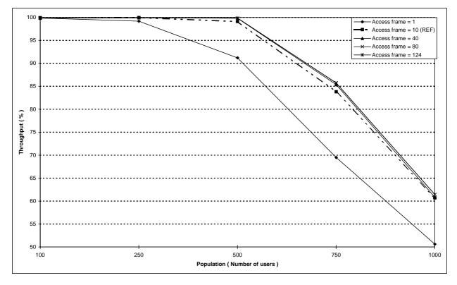
Figure 116: Individual M-M circuit switched call set-up throughput versus number of users for different values of the random access frame length
