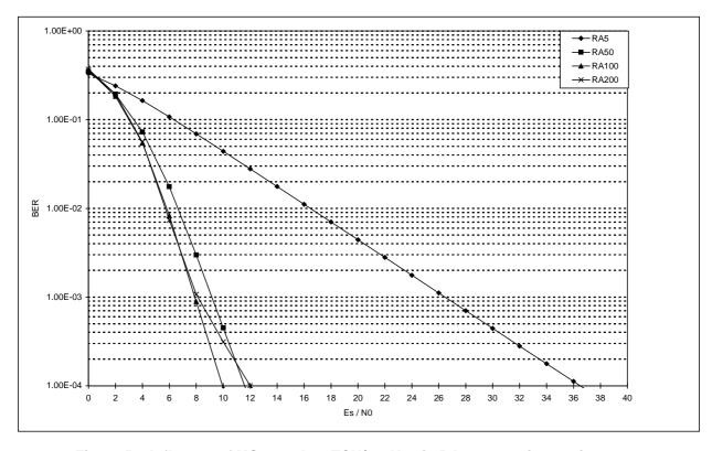
Figure 58: Influence of MS speed on TCH/2,4 N=4 in RA propagation environment
