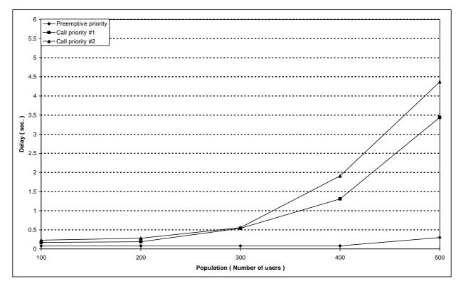
Figure 188: Individual M-M circuit switched call set-up  $\tau_{95\%}$  boundary delay versus number of users in a cell with 11 TCHs allocated
