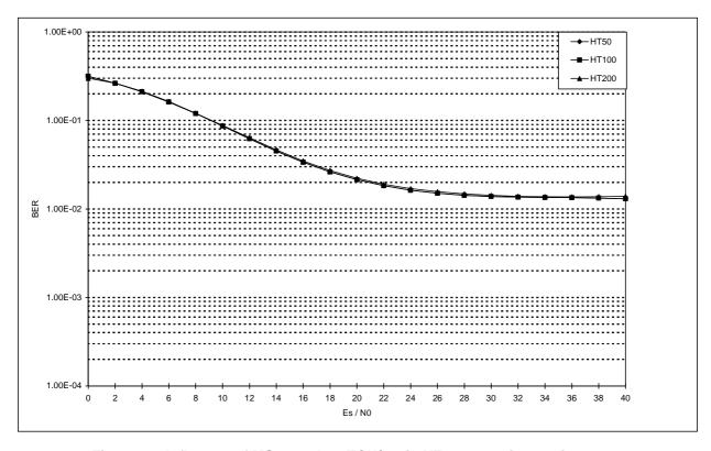
Figure 29: Influence of MS speed on TCH/7,2 in HT propagation environment
