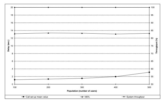
Figure 171: Individual M-M packet data call set-up performance versus number of users for priority distribution B
