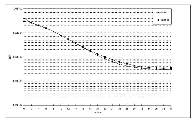
Figure 27: Influence of MS speed on TCH/7,2 in BU propagation environment
