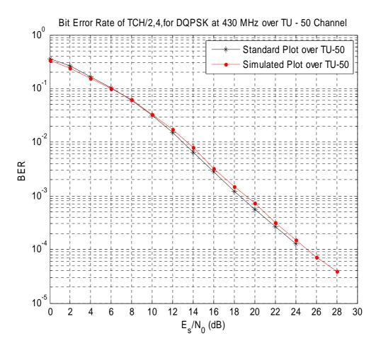
Figure G.7: Bit Error Rate of TCH/2,4 over TU50 propagation channel for 430 MHz, results corresponds to figure 50 of clause 4.4
