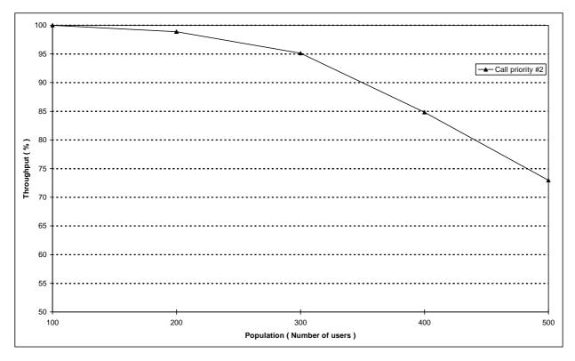
Figure 166: Individual M-M circuit switched call set-up system throughput versus number of users for priority distribution A
