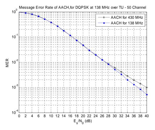
Figure F.5: Message Error Rate of AACH over TU50 Propagation Channel for 138 MHz
