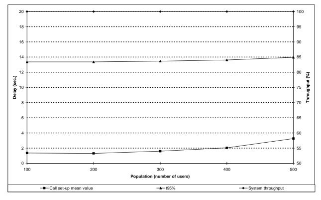
Figure 156: Individual M-M packet data call set-up performance versus number of users for scenario 8D (Reference with radio Dispatcher)
