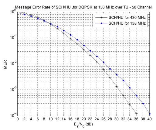
Figure F.8: Message Error Rate of SCH/HU over TU50 Propagation Channel for 138 MHz
