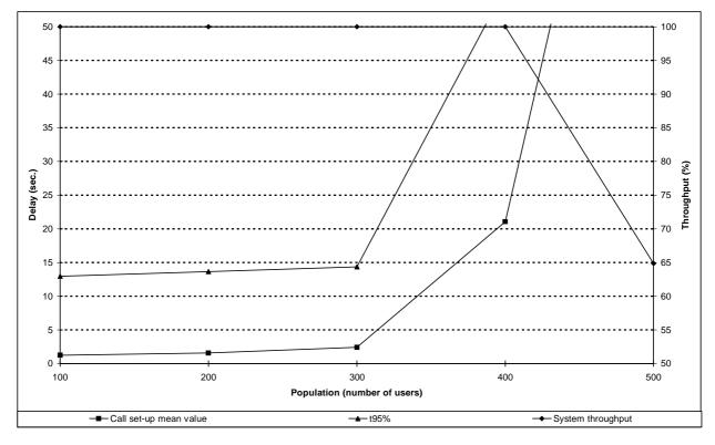
Figure 148: Individual M-M packet data call set-up performance versus number of users for scenario 8B (Packet data generation rate = 15/h)
