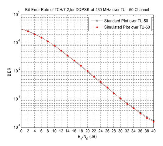
Figure G.6: Bit Error Rate of TCH/7,2 over TU-50 propagation channel for 430 MHz, results corresponds to figure 26 of clause 4.4
