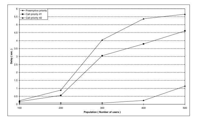
Figure 139: Individual M-M circuit switched call set-up  $\tau_{95\%}$  boundary delay versus number of users for the reference configuration
