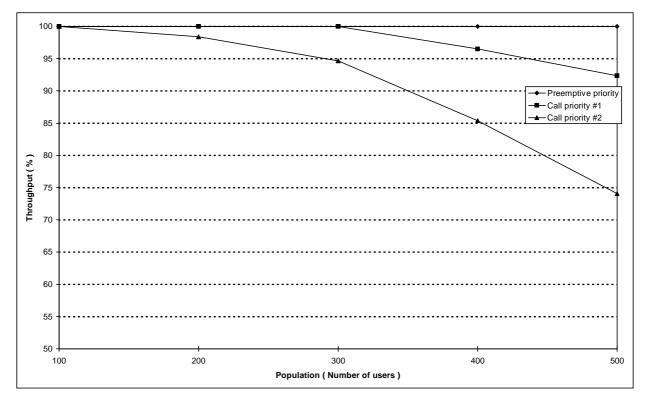
Figure 140: Individual M-M circuit switched call set-up system throughput versus number of users for the reference scenario
