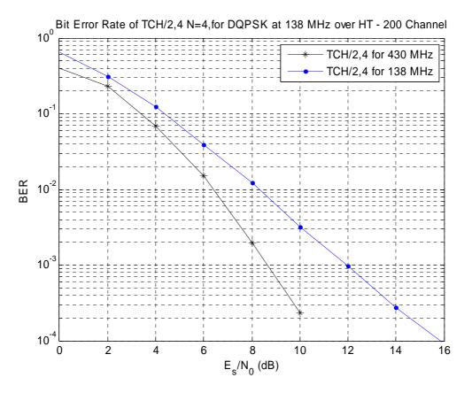
Figure F.22: Bit Error Rate of TCH/2,4 N=4 over HT200 Propagation Channel for 138 MHz
