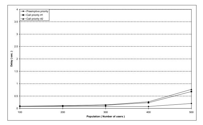
Figure 187: Individual M-M circuit switched call set-up mean delay versus number of in a cell with 11 TCHs allocated
