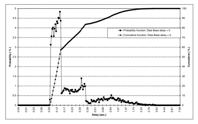
Figure 75: Probability function and cumulative distribution of call set-up time with zero delay data base
