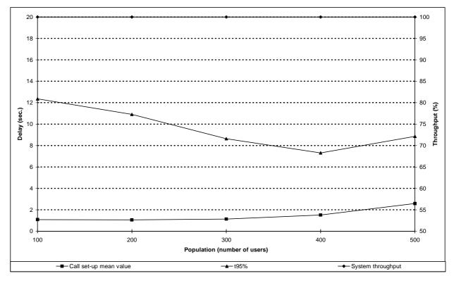
Figure 186: Individual M-M packet data call set-up performance versus number of users in a cell with 3 TCHs allocated
