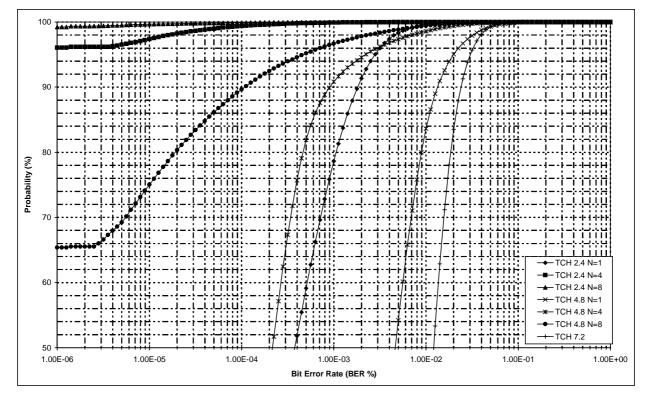
Figure 199: BER versus probability for different traffic channels in BU100 propagation environment
