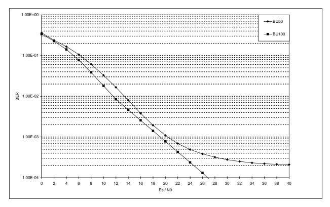
Figure 51: Influence of MS speed on TCH/2,4 N=1 in BU propagation environment
