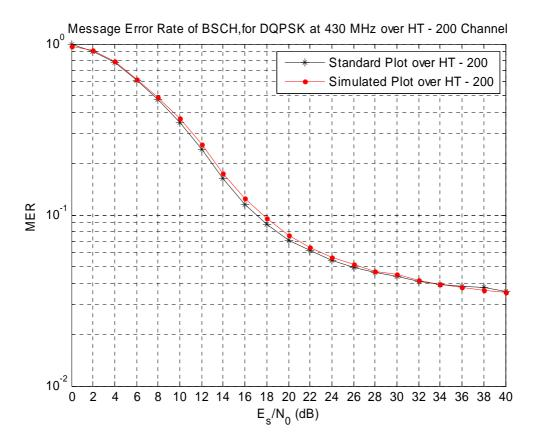
Figure G.14: Message Error Rate of BSCH Channel over HT200 propagation channel for 430 MHz, results corresponds to figure 24 of clause 4.3
