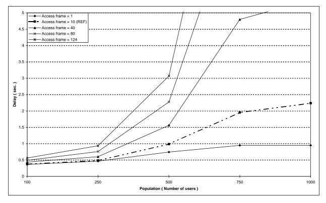
Figure 118: Individual M-F short data transmission mean delay versus number of users for different values of the random access frame length
