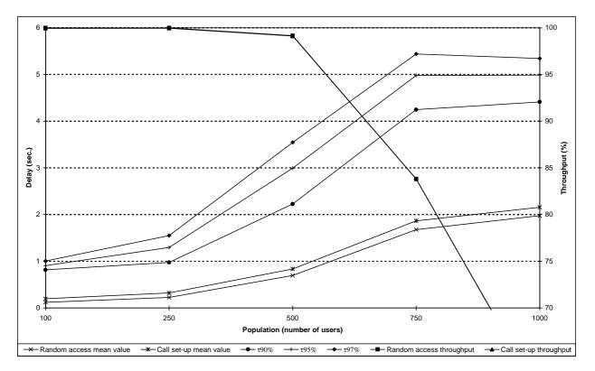
Figure 91: Individual M-M voice or circuit data call performance for scenario 1D (reference) (throughput curves overlap)
