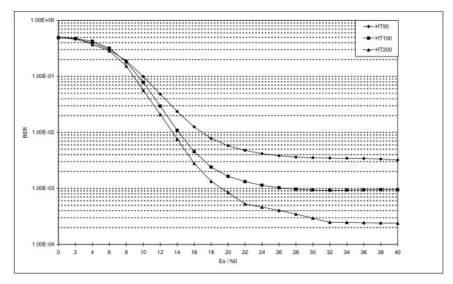
Figure 41: Influence of MS speed on TCH/4,8 N=4 in HT propagation environment
