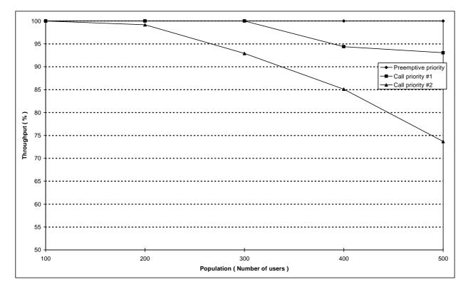
Figure 147: Individual M-M circuit switched call set-up system throughput versus number of users for scenario 8B (Packet data generation rate = 15/h)
