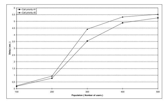
Figure 173: Individual M-M circuit switched call set-up  $\tau_{95\%}$  boundary delay versus number of users for priority distribution C
