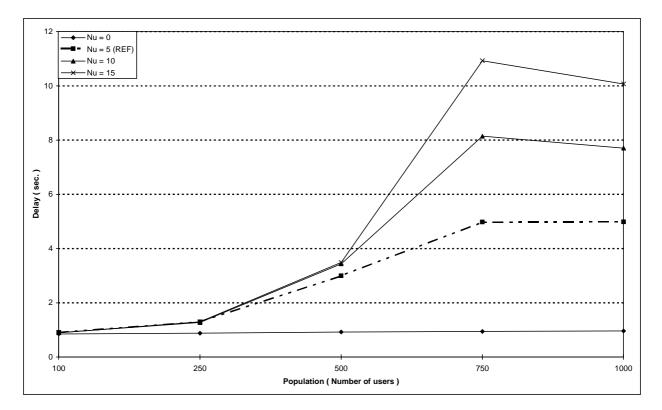
Figure 109: Individual M-M circuit switched call set-up τ<sub>95 %</sub> boundary delay versus number of users for different values of the maximum number of re-transmissions in the random access Nu
