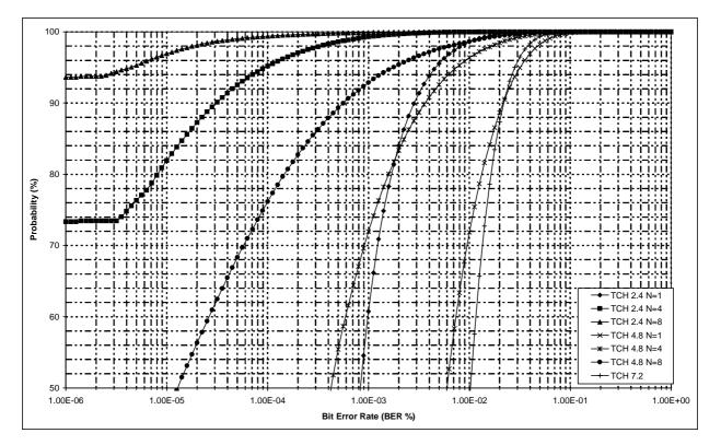
Figure 198: BER versus probability for different traffic channels in BU50 propagation environment
