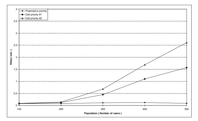
Figure 153: Individual M-M circuit switched call set-up mean delay versus number of users for scenario 8D (Reference with radio Dispatcher)
