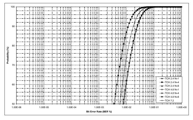
Figure 195: BER versus probability for different traffic channels in TU5 propagation environment
