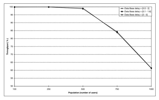
Figure 84: Comparison of call set-up throughput for different characteristics of system data base (all curves overlap)
