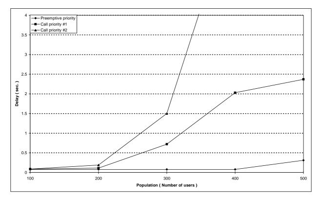
Figure 191: Individual M-M circuit switched call set-up mean delay versus number of users with maximum hold time in priority queue = 300 TDMA frames
