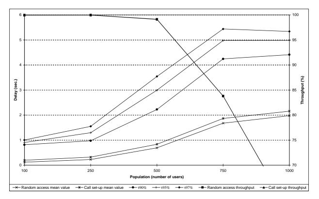
Figure 95: Individual M-M voice or circuit data call performance for the reference scenario (throughput curves overlap)
