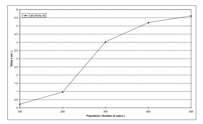
Figure 165: Individual M-M circuit switched call set-up  $\tau_{95\%}$  boundary delay versus number of users for priority distribution A
