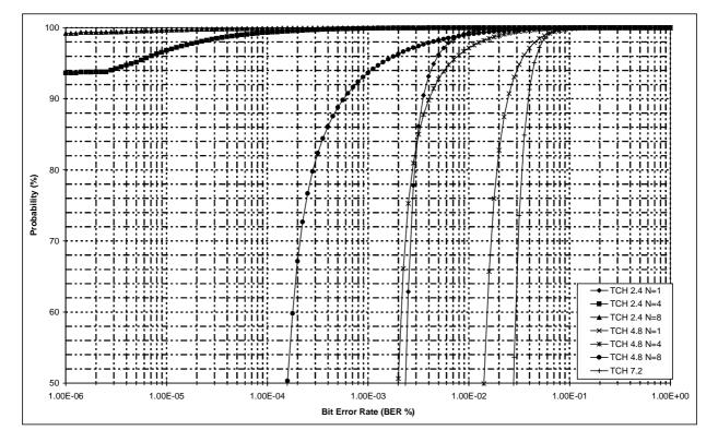
Figure 205: BER versus probability for different traffic channels in HT 100 propagation environment
