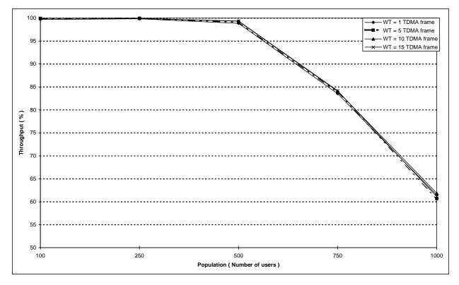
Figure 100: Individual M-M circuit switched call set-up throughput versus number of users for different values of the retransmission timer WT (all curves overlap)
