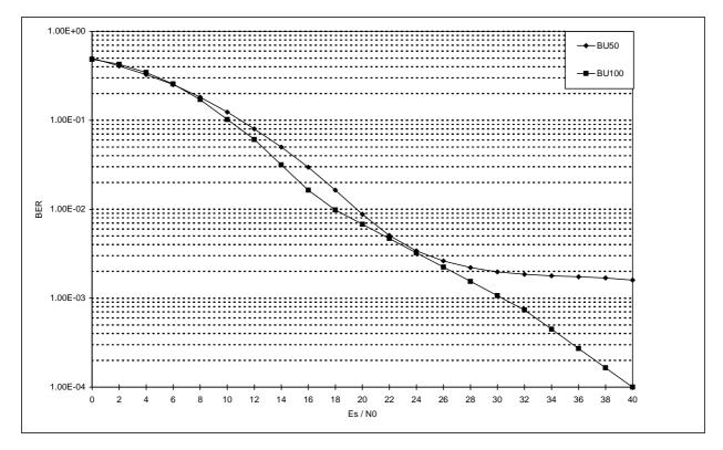
Figure 33: Influence of MS speed on TCH/4,8 N=1 in BU propagation environment
