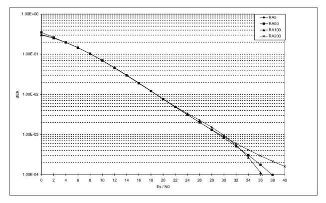
Figure 28: Influence of MS speed on TCH/7,2 in RA propagation environment
