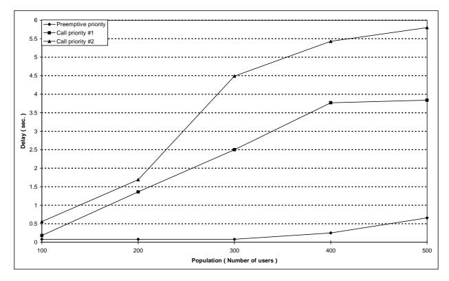
Figure 150: Individual M-M circuit switched call set-up  $\tau_{95\%}$  boundary delay versus number of users for scenario 8C (Packet data generation rate = 30/h)
