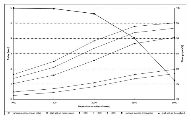
Figure 86: Individual M-F short data transmission performance for scenario 1A (throughput curves overlap)
