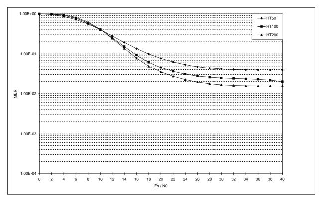
Figure 18: Influence of MS speed on SCH/F in HT propagation environment
