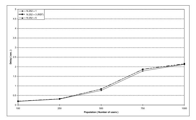
Figure 123: Individual M-M circuit switched call set-up mean delay versus number of users for different values of the basic link maximum number of re-transmissions
