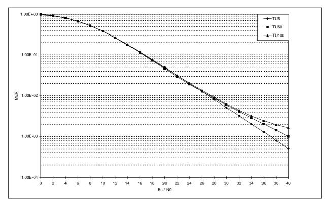
Figure 3: Influence of MS speed on AACH in TU propagation environment
