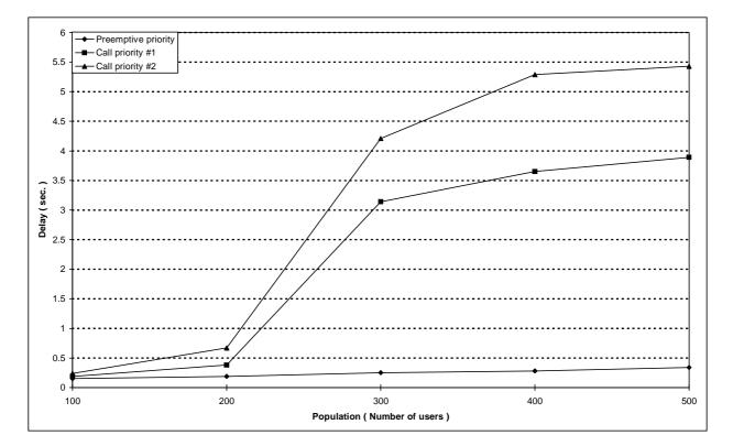
Figure 143: Dispatcher to Mobile group call set-up  $\tau_{95\%}$  boundary delay versus number of users for the reference configuration
