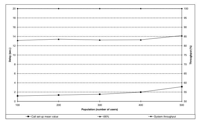
Figure 141: Individual M-M packet data call set-up performance versus number of users for the reference scenario
