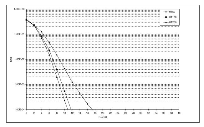
Figure 59: Influence of MS speed on TCH/2,4 N=4 in HT propagation environment
