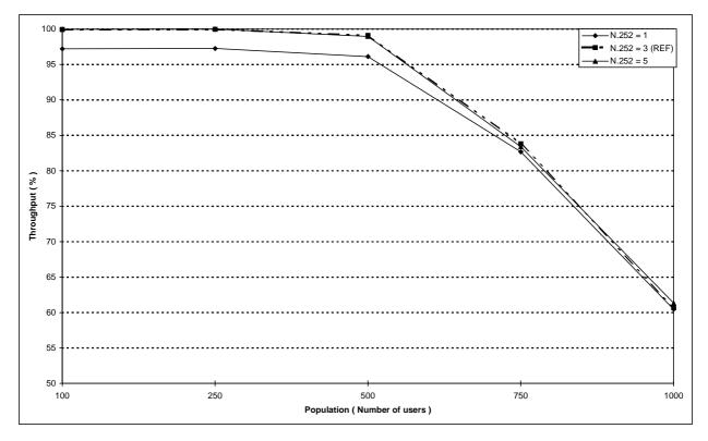
Figure 124: Individual M-M circuit switched call set-up throughput versus number of users for different values of the basic link maximum number of re-transmissions
