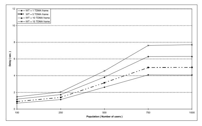
Figure 104: Individual M-F short data transmission  $\tau_{95\,\%}$  boundary delay versus number of users for different values of the retransmission timer WT
