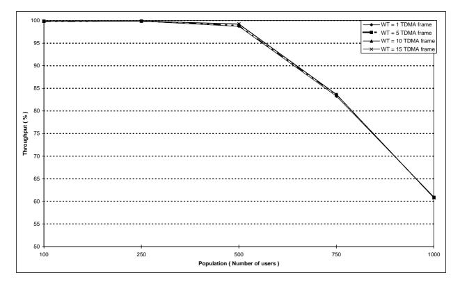
Figure 103: Individual M-F short data transmission throughput versus number of users for different values of the retransmission timer WT (all curves overlap)
