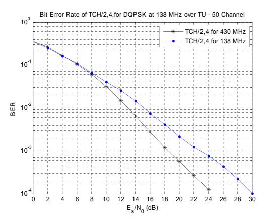
Figure F.10: Bit Error Rate of TCH/2,4 over TU50 Propagation Channel for 138 MHz
