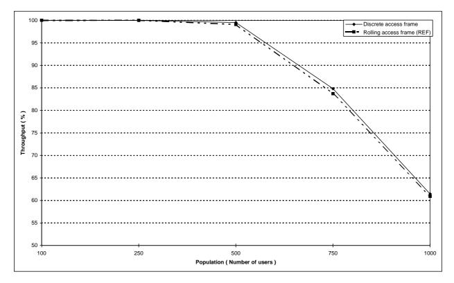
Figure 130: Random access throughput versus number of users for different access techniques
