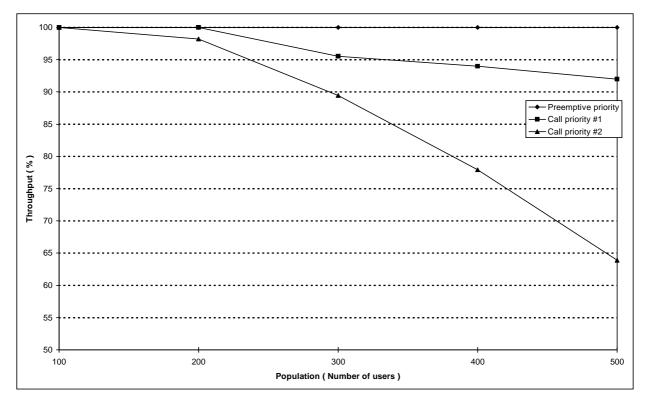
Figure 181: Individual M-F circuit switched call set-up system throughput versus number of users in case of full duplex circuit calls
