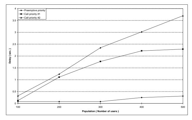
Figure 183: Individual M-M circuit switched call set-up mean delay versus number of users in a cell with 3 TCHs allocated
