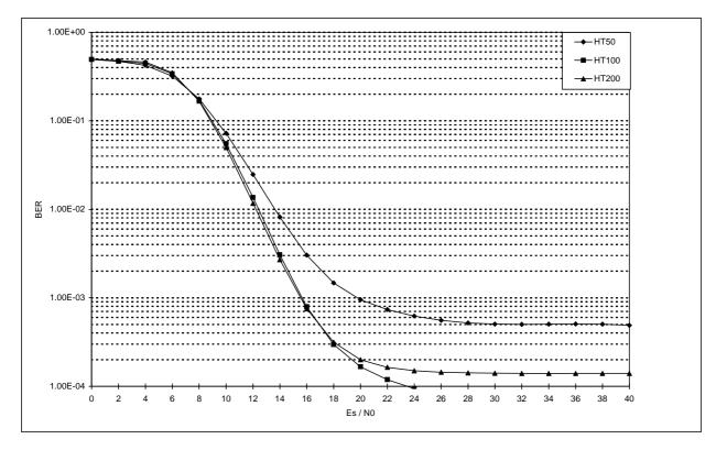
Figure 47: Influence of MS speed on TCH/4,8 N=8 in HT propagation environment
