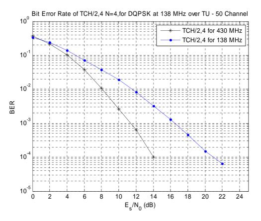
Figure F.11: Bit Error Rate of TCH/2,4 N=4 over TU50 Propagation Channel for 138 MHz
