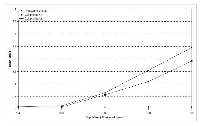
Figure 138: Individual M-M circuit switched call set-up mean delay versus number of users for the reference configuration
