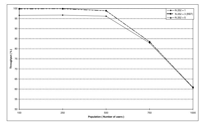
Figure 127: Individual M-F short data transmission throughput versus number of users for different values of the basic link maximum number of re-transmissions
