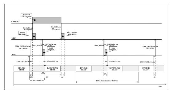
Figure 69: Time diagram related to message exchange in MAC, LLC and layer 3 with long response times
