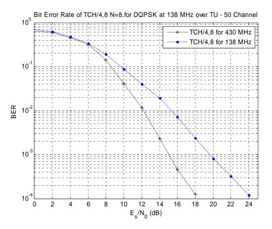
Figure F.15: Bit Error Rate of TCH/4,8 N=8 over TU50 Propagation Channel for 138 MHz
