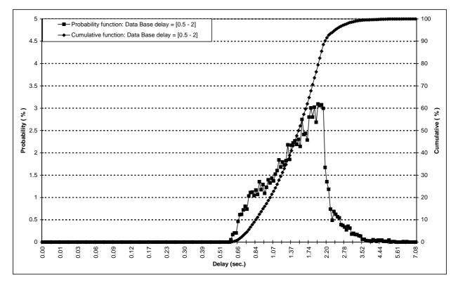
Figure 77: Probability function and cumulative distribution of call set-up time with data base delay uniformly distributed between 0,5 s and 2 s
