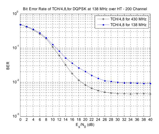
Figure F.24: Bit Error Rate of TCH/4,8 over HT200 Propagation Channel for 138 MHz
