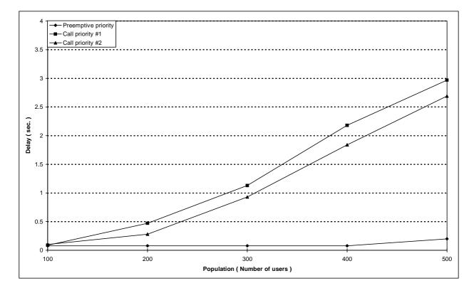
Figure 176: Individual M-M circuit switched call set-up mean delay versus number of users in case of full duplex circuit calls
