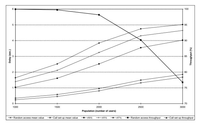
Figure 85: Individual M-M voice or circuit data call performance for scenario 1A (throughput curves overlap)
