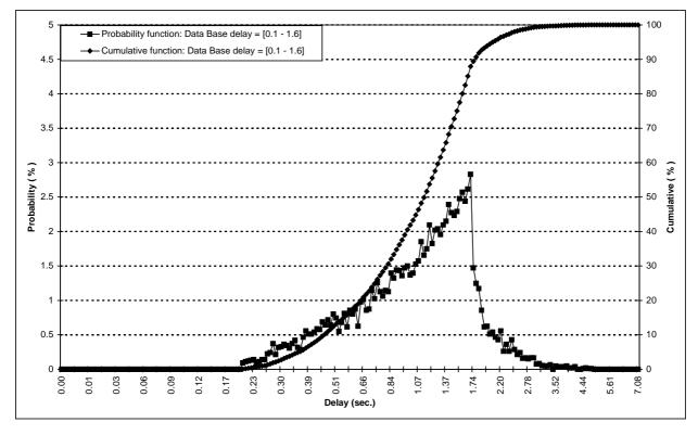
Figure 76: Probability function and cumulative distribution of call set-up time with data base delay uniformly distributed between 0,1 s and 1,6 s
