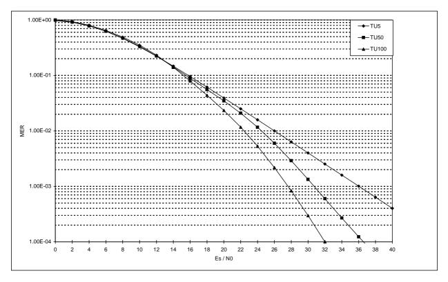
Figure 9: Influence of MS speed on SCH/HU in TU propagation environment
