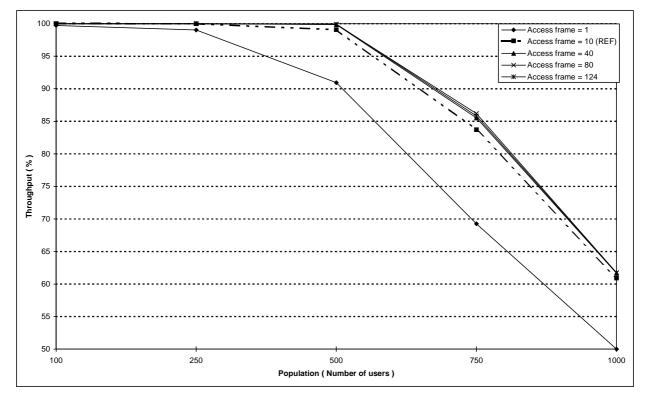
Figure 114: Random access throughput versus number of users for different values of the random access frame length
