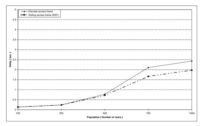
Figure 129: Random access mean delay versus number of users for different access techniques
