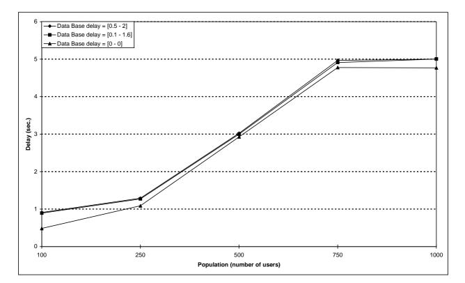
Figure 81: Comparison of call set-up τ<sub>95 %</sub> for different characteristics of system data base (curves for delay in 0,5 s to 2 s and in 0,1 s to 1,6 s overlap)
