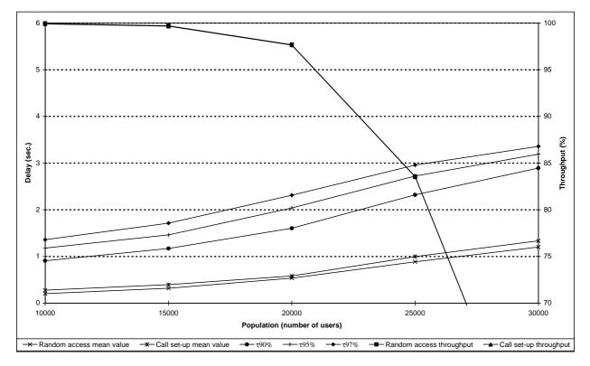
Figure 93: Individual M-M voice or circuit data call performance for scenario 1E (throughput curves overlap)
