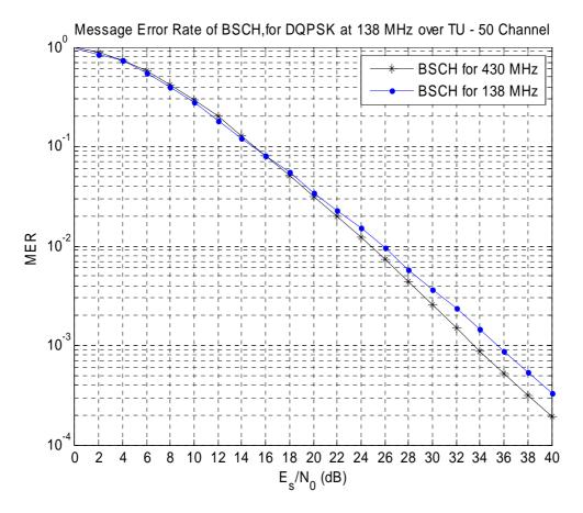
Figure F.6: Message Error Rate of BSCH over TU50 Propagation Channel for 138 MHz
