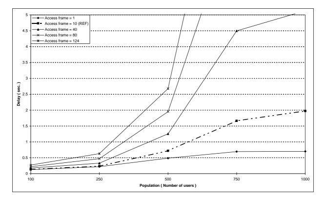
Figure 113: Random access mean delay versus number of users for different values of the random access frame length
