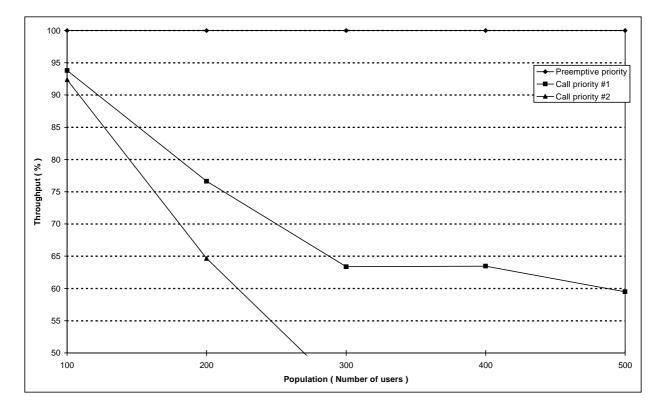
Figure 185: Individual M-M circuit switched call set-up system throughput versus number of users in a cell with 3 TCHs allocated
