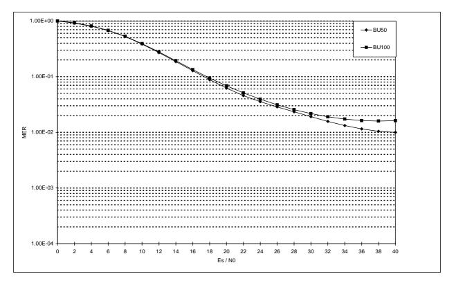
Figure 4: Influence of MS speed on AACH in BU propagation environment
