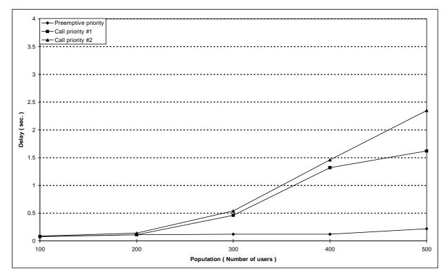
Figure 168: Individual M-M circuit switched call set-up mean delay versus number of users for priority distribution B
