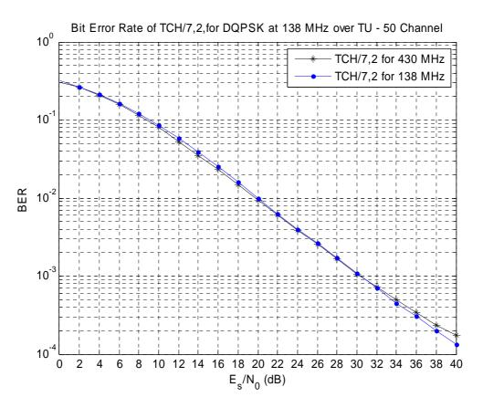
Figure F.9: Bit Error Rate of TCH/7,2 over TU50 Propagation Channel for 138 MHz
