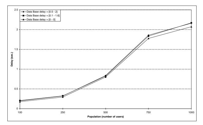
Figure 79: Comparison of call set-up mean value for different characteristics of system data base (curves for delay in 0,5 s to 2 s and in 0,1 s to 1,6 s overlap)
