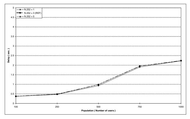
Figure 126: Individual M-F short data transmission mean delay versus number of users for different values of the basic link maximum number of re-transmissions
