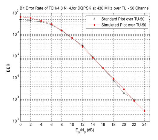
Figure G.11: Bit Error Rate of TCH/4,8 N=4 over TU50 propagation channel for 430 MHz, results corresponds to figure 38 of clause 4.4
