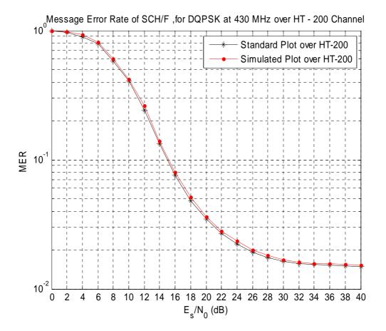
Figure G.15: Message Error Rate of SCH/F Channel over HT200 propagation channel for 430 MHz, results corresponds to figure 18 of clause 4.3
