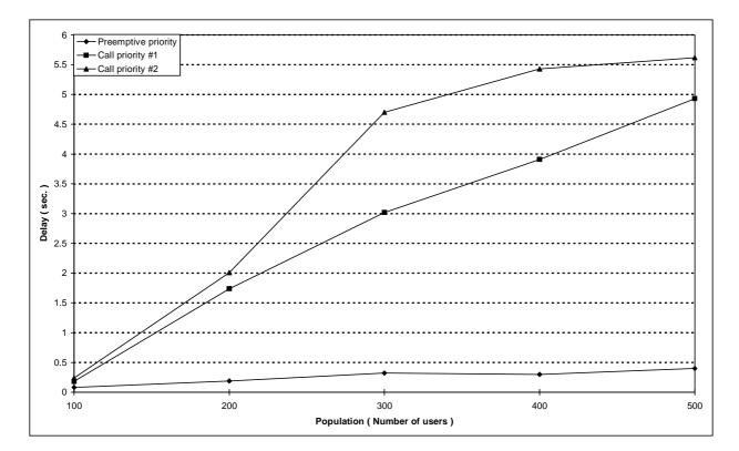
Figure 180: Individual M-F circuit switched call set-up  $\tau_{95\,\%}$  boundary delay versus number of users in case of full duplex circuit calls
