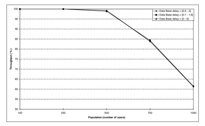
Figure 83: Comparison of random access throughput for different characteristics of system data base (all curves overlap)
