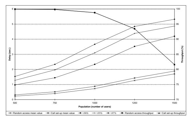
Figure 87: Individual M-M voice or circuit data call performance for scenario 1B (throughput curves overlap)
