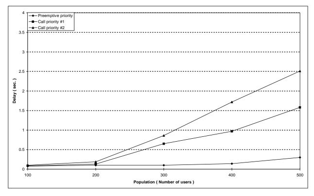
Figure 179: Individual M-F circuit switched call set-up mean delay versus number of users (full duplex calls)
