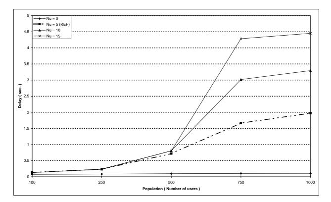
Figure 105: Random access mean delay versus number of users for different values of the maximum number of re-transmissions in the random access Nu
