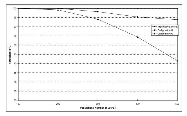
Figure 151: Individual M-M circuit switched call set-up system throughput versus number of users for scenario 8C (Packet data generation rate = 30/h)
