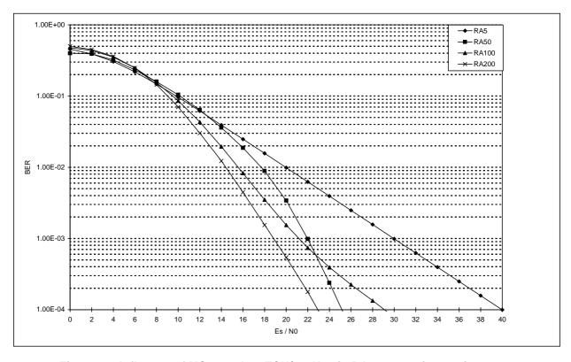
Figure 34: Influence of MS speed on TCH/4,8 N=1 in RA propagation environment
