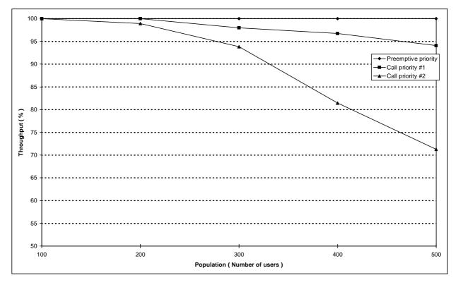
Figure 170: Individual M-M circuit switched call set-up system throughput versus number of users for priority distribution B
