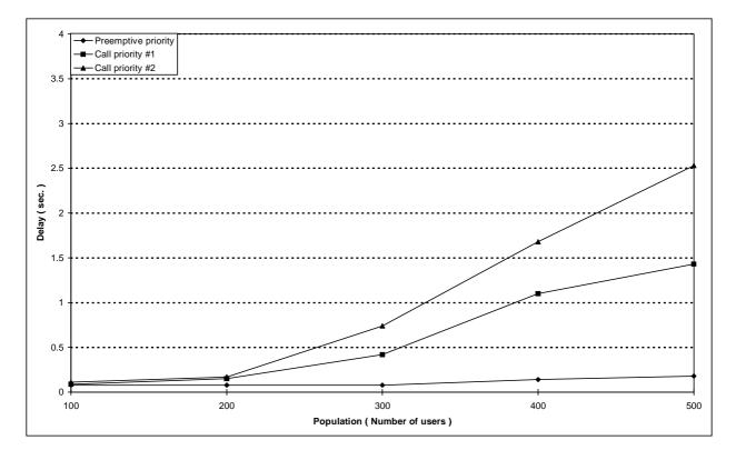
Figure 145: Individual M-M circuit switched call set-up mean delay versus number of users for scenario 8B (Packet Data generation rate = 15/h)
