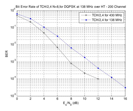
Figure F.23: Bit Error Rate of TCH/2,4 N=8 over HT200 Propagation Channel for 138 MHz
