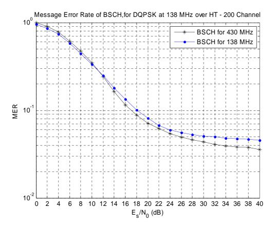
Figure F.17: Message Error Rate of BSCH over HT200 Propagation Channel for 138 MHz
