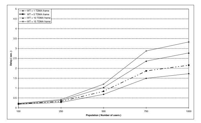
Figure 99: Individual M-M circuit switched call set-up mean delay versus number of users for different values of the retransmission timer WT
