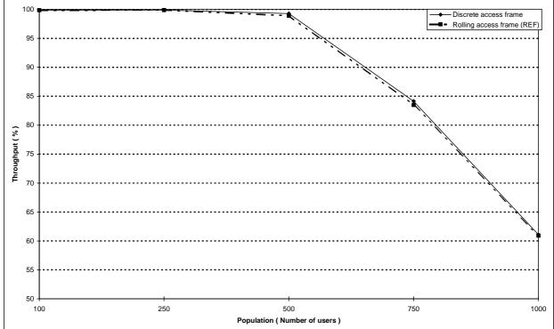
Figure 135: Individual M-F short data transmission throughput versus number of users for different access techniques
