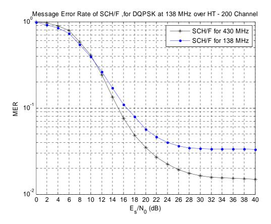
Figure F.18: Message Error Rate of SCH/F over HT200 Propagation Channel for 138 MHz
