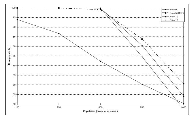
Figure 108: Individual M-M circuit switched call set-up throughput versus number of users for different values of the maximum number of re-transmissions in the random access Nu
