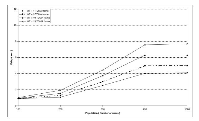
Figure 101: Individual M-M circuit switched call set-up  $\tau_{95\%}$  boundary delay versus number of users for different values of the retransmission timer WT
