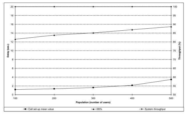
Figure 190: Individual M-M packet data call set-up performance versus number of users in a cell with 11 TCHs allocated
