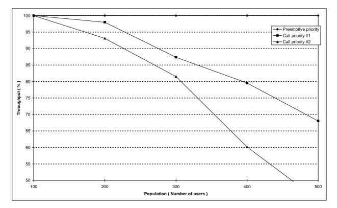
Figure 178: Individual M-M circuit switched call set-up system throughput versus number of users in case of full duplex circuit calls
