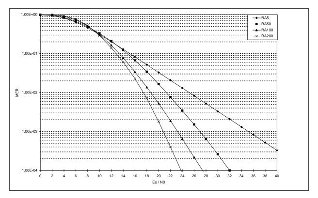
Figure 17: Influence of MS speed on SCH/F in RA propagation environment
