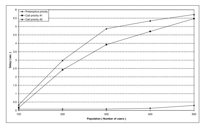
Figure 177: Individual M-M circuit switched call set-up  $\tau_{95\%}$  boundary delay versus number of users in case of full duplex circuit calls
