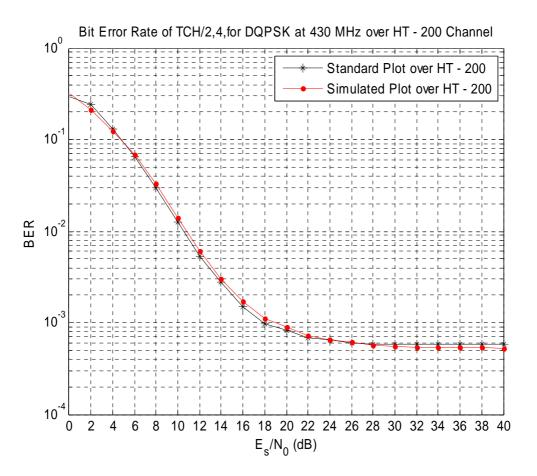
Figure G.18: Bit Error Rate of TCH/2,4 Channel over HT200 propagation channel for 430 MHz, results corresponds to figure 53 of clause 4.4
