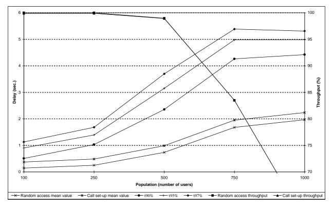
Figure 96: Individual M-F short data transmission performance for the reference scenario (throughput curves overlap)
