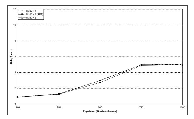
Figure 125: Individual M-M circuit switched call set-up τ<sub>95 %</sub> boundary delay versus number of users for different values of the basic link maximum number of re-transmissions
