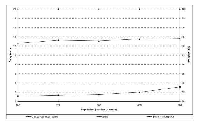
Figure 175: Individual M-M packet data call set-up performance versus number of users for priority distribution C
